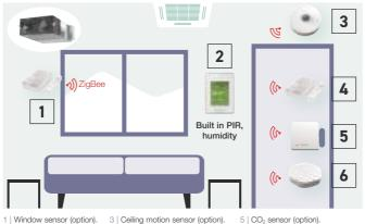
1 | Window sensor (option). 2 | Room controller. 3 | Ceiling motion sensor (option). 4 | Door sensor (option). 5 | CO<sub>2</sub> sensor (option). 6 | Water leakage sensor (option).
