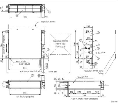
1 Refrigerant piping joint (narrow tube) 2 Refrigerant piping joint (wide tube) 3 Upper and bottom drain port (O.D. 26 mm) 4 Suspension lug 5 Power supply outlet (2- Ø30) 6 Flange for air intake duct 7 Pl cover 8 Electrical component box 9 Frame filter
