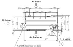
When using a drain pipe, install the drain socket (field supply) on to the drain port.Seal the other drain port with the rubber cap.
