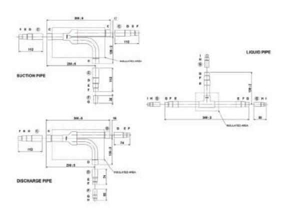
All measurements are in mm. Size of connection points on each part shown are inside diameters of piping.
