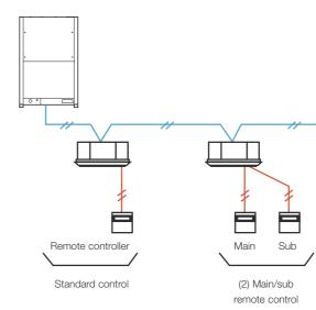
NOTE: Connectable number of controllers, controller combination, connectable indoor units, remote control maximum wiring lengh are different between the controller. Please confirm the installation Instructions of controller or consult with Panasonic service center.
