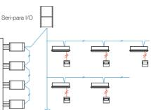
• This unit can control up to 4 outdoor units. • From the centre control device, mode changing and batch operation/batch stop are possible. • Required for demand control.
