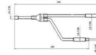
All measurements are in mm. Size of connection points on each part shown are inside diameters of piping.
