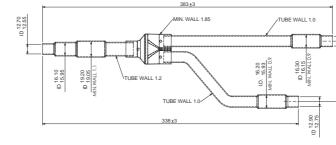
All measurements are in mm. Size of connection points on each part shown are inside diameters of piping.
