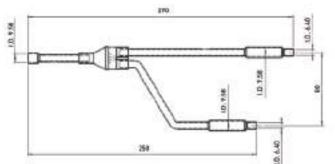
All measurements are in mm. Size of connection points on each part shown are inside diameters of piping.
