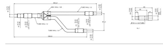
All measurements are in mm. Size of connection points on each part shown are inside diameters of piping.
