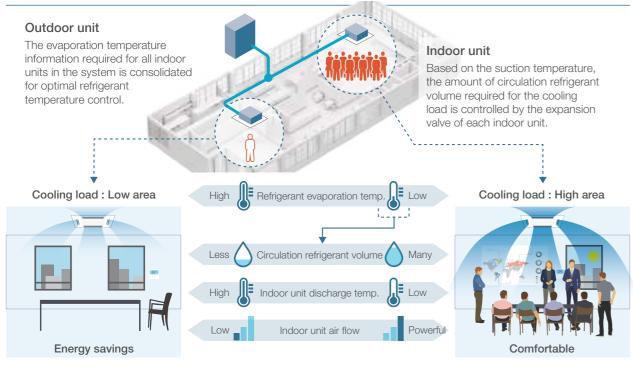
Combination of VET technology and inverter compressor achieves both energy savings and comfort by smoothly controlling the compressor to match the air conditioning load without stopping the compressor for optimum performance.
