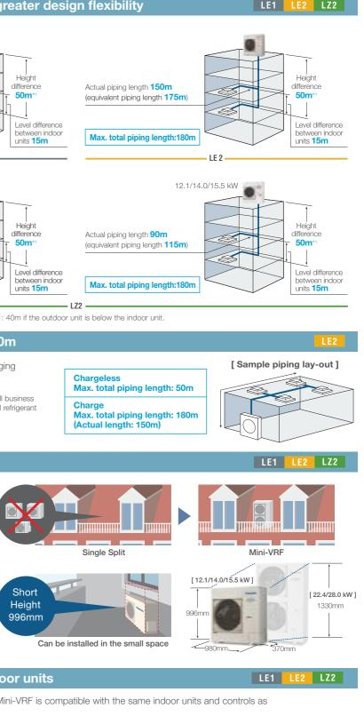
In addition to raising efficiency, we have made the outdoor unit more compact. It can now be installed in places that were previously too small.
