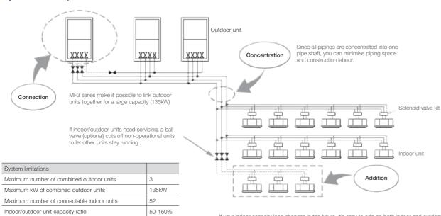
If your indoor capacity load changes in the future, it's easy to add on both indoor and outdoor units using the same pipings.
